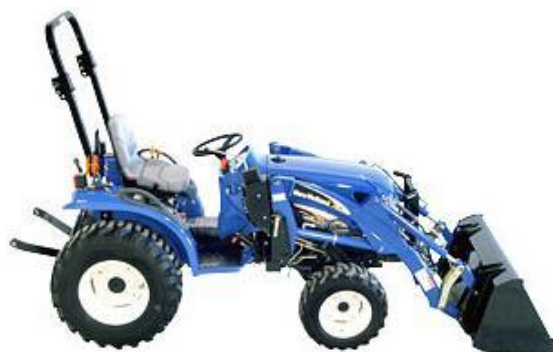
T1110 New Holland 4x4 Compact Tractor, with 210 Quick Attach Loader and 48" Bucket.
